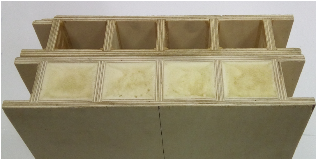
Figure 4. Sandwich panel initial prototype with and without polyurethane foam.
