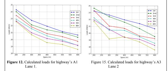
In this study comprehensive WIM data cleaning was performed based on four different types of filters. Then cleaned data were used to calculate uniformly distributed loads for 200, 300, 400, 500, 600 meters long bridges spans were calculated.
