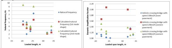
Fig.1 Natural frequency dependence on loaded Fig.2 DAF dependence on loaded length
